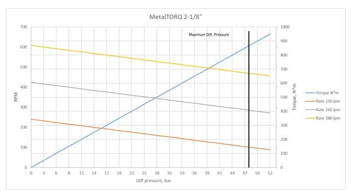
Operational specifications are for reference only. Actual tool performance may vary depending on a variety of downhole conditions. Performance data based upon standard conditionals with fresh water in a controlled setting. Some amount of liquid must be pump during operations with N2. Terms such as "Stall Diff. Pressure & Stall Torque" cannot be applied based on data with conventional PDMs.
